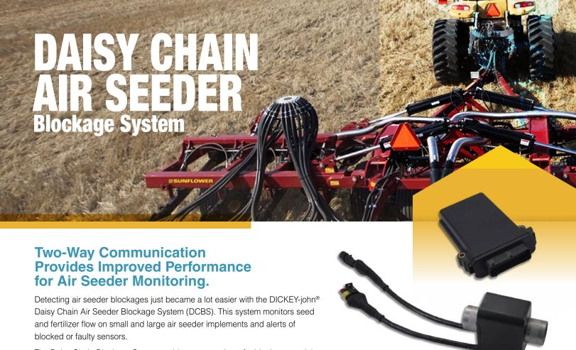
The Daisy Chain Blockage System architecture consists of a blockage module and daisy chain (serial communication) blockage sensors. Each module and sensor displays on the virtual terminal indicating critical system parameters for the selected loop.
