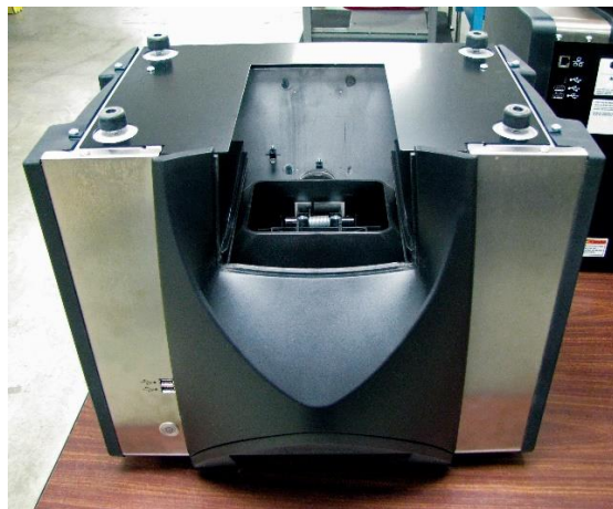
Figure 14 Place Instrument Upside Down
