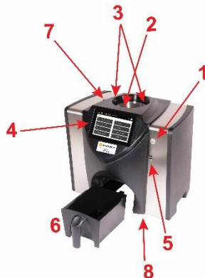
Figure 1 GAC™ 2700-UGMA Moisture Tester Overview (Front of Unit)
