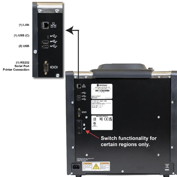
Figure 2 External Communication Connections (Back of Unit)
