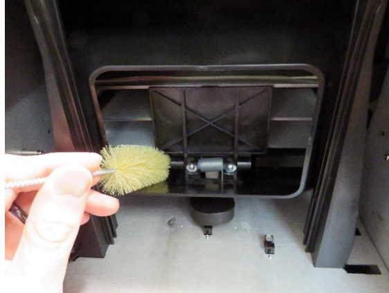
Figure 12 Clean Under Trap Door
